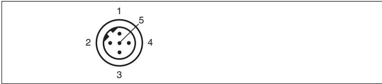
Figure 4.5 Profibus Bus In connection layout
