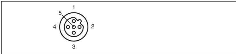
Figure 4.8 Interbus Remote Bus Out connection layout
