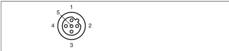
Figure 4.6 Profibus Bus Out and Termination connection layout
